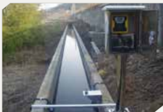
Laser Pointer Tool used to adjust transducer angle(patented)
